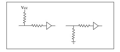
Figure 5.7 Ultra DMA termination with pull-up or pull-down
